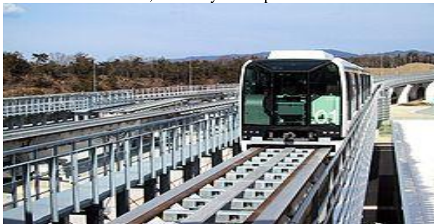
Railroad with vehicle on air cushion
