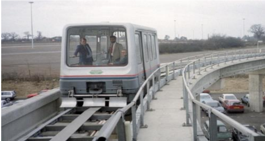
Rail track with linear electric motor
